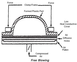
A simple suction or blowing mold consists of a base plate with a clamping frame. Enough mechanical or hydraulic toggle clamps must be provided to maintain frame rigidity and to withstand the forming pressure. Using screw clamps has the disadvantage of being time consuming and may allow the sheet to cool excessively before it is formed. Beaded clamping frames will seal better than flat frames.
