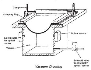
Resting the sheet blank on a cold base plate may cause undesired cooling while installing the clamping frame. To reduce this heat the plate or cover it with thick, nonlinting cloth.
