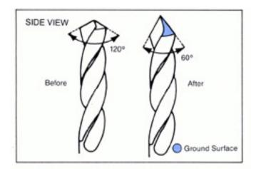
The cutting edge must be ground "flat" to a 0-4° rake angle. This cutting edge will scrape the acrylic, not gouge it.
