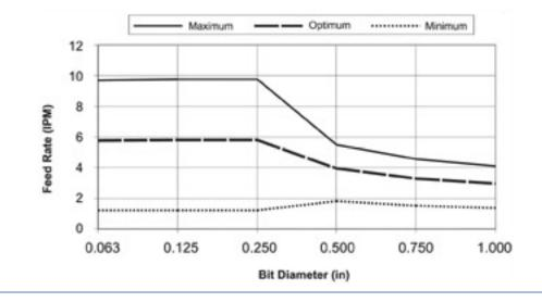
As indicated in the graphs and table above, lower SFM's are required for larger drill bits. This is to ensure smooth, vibration-free drilling because large bits will tend to grab the material more. As a result, feed rate must generally be slowed down in order to prevent chipping and consequently spindle speed must be reduced to prevent melting.
