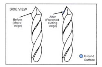
The surface behind the cutting edge must be ground away to clearance angles of 12-15°. This back relief reduces metal/plastic contact and heat build-up. This modification is standard on most high quality twist drill bits.
