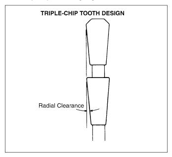
Best results are achieved when the teeth have a clearance angle (top clearance) of 10° to 15°. This minimizes contact between the teeth and the material reducing friction and resulting in less melting. The proper rake or "hook" angle, 0° to 5° positive, ensures the teeth do not strike the material too aggressively. Higher angles can lead to chipping due to poor blade stability and poor control of material feed rates.
