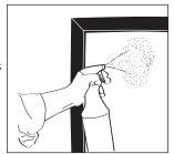
Apply Film In Place with the adhesive side on the window. The soap solution acts as a lubricant to allow positioning of film. GENEROUSLY spray "room-side" surface of film to lubricate before squeegeeing.
