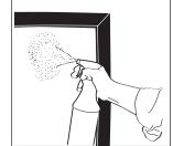
Clean Finished Window with a non-ammoniated window cleaner (your soap-solution is ideal). When you clean the window, be careful not to disturb the film's adhesion to the glass—it will not bond completely until it is dry, which can take up to 30 days depending on sun exposure.
