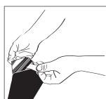
Spray Soap Solution generously over entire window surface. Avoid spraying the edge of the glass as this can wash trapped dirt onto the glass. Next spray adhesive side of film with the soap solution (the side exposed by removal of liner).
