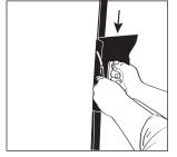
window together. This will trim the film in a straight line and leave a <sup>1</sup>/16" gap between the film and the window frame. Repeat for the other edges.
