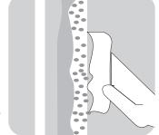
Begin buffing immediately with a power buffer. It is recommended that the power buffer be equipped with a terry cloth or cotton pad.
