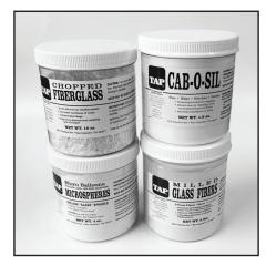
Thickened resin can be used for hole/gap filling, filleting, and bonding porous and nonporous objects. See below for bonding instructions. Cab-O-Sil creates an extremely hard, somewhat brittle, abrasion-resistant surface. Cured resin with Cab-O-Sil is very difficult to sand, so use care in application to avoid sanding problems. Combine with Microspheres to create a putty-like mixture for sanding.
