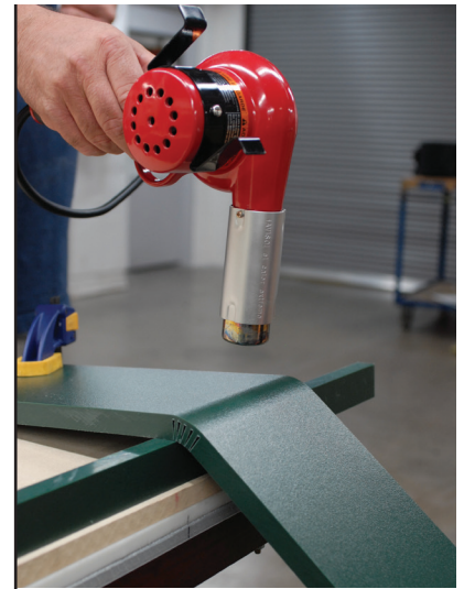
A bending bar can be used to produce a tight radius.
