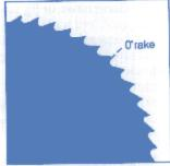
For circular saws, use a metal cutting blade—not a combination blade.
