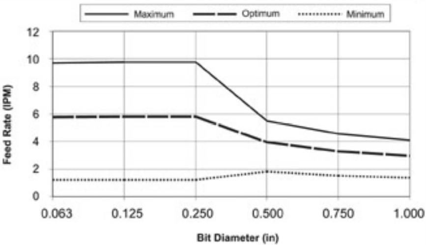
As indicated in the graphs and table above, lower SFM's are required for larger drill bits. This is to ensure smooth, vibration-free drilling because large bits will tend to grab the material more. As a result, feed rate must generally be slowed down in order to prevent chipping and consequently spindle speed must be reduced to prevent melting.
