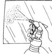
**3** **REMOVE** clear protective liner by attaching masking tape to front and back surfaces of one corner. Pull tape apart and the clear film will separate to expose the adhesive. Immediately spray the exposed adhesive with the soap and water solution to avoid dust adhering to surface. Spray your fingertips before handling adhesive surface. Spray window again and make it dripping wet.
