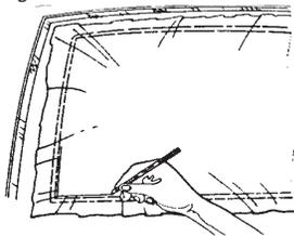
If it is not possible to cut the film to the exact window size, then cut to a rough size approximately 1/2" wider and 1/2" longer than needed. Do one window at a time. Make final trim after applying film to each window.
