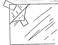
**4** **PLACE** wet surface of the film (adhesive side against the window) upon the wet inside surface of the window. Film can be moved or slipped easily into position. Handle film carefully to avoid scratching or creasing. (Air bubbles can be removed with the squeegee, but creases cannot.)
