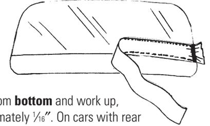
**8** **CUT A PATTERN** for entire window and use it for cutting strips. Strips should be 1/16" to 1/8" wider than the pattern to allow for overlap. Use normal installation procedures as described earlier and exercise caution when squeegeeing over the seams.
