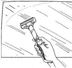
**NOT USE a razor blade over defroster lines, as this may damage them, instead clean with a WHITE Scrunge or Dobie pad** (made specifically for scouring Teflon). Clean with lint-free towels. If small particles are trapped between glass and film they appear as white bubbles that never disappear. Meticulous cleaning is mandatory for a good-looking, long-lasting installation. Wash outside surface of windows also.
