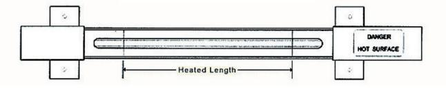
All Free-Standing Heating Trays run on standard 120 volts and have a maximum operating temperature of 800°f. Units can be used with below listed Power Controls where temperature control is desired.
