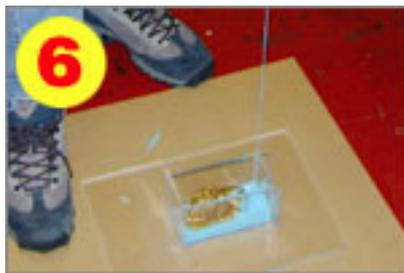
As in #4 above, pour into the corner of the mold and allow the silicone to 'squeegee' air out ahead of it, to minimize trapped bubbles.
