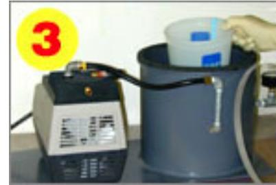
Mixed silicone will be loaded with bubbles (if it is mixed properly). These bubbles can ruin a mold if they are anywhere near the surface of the part. There are two ways to minimize bubbles. The vacuum chamber, pictured here is one method, and step five describes the other.
