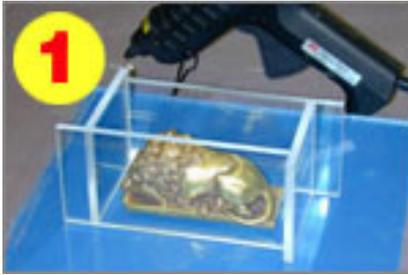
Find or make a container to hold your original part. Container must be leak proof. Construct the container so that the mold walls will be approximately 1/2" thick. Walls thicker than 1/2" make a mold difficult to work with and use more material. Under 1/2" causes the mold to deform when filled with resin.
