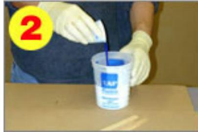
Measure the catalyst and silicone, 10 parts silicone to 1 part catalyst by volume. THOROUGHLY mix until there are no streaks. Look at the outside and bottom of the transparent mixing cup. If it is white, more mixing is required. This step cannot be over emphasized! Incomplete mixing will yield inferior results.
