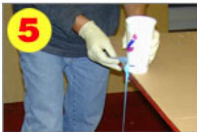
If you do not have a vacuum chamber, there is another method to minimize air in the mold. Cut a 1/2" diameter hole in the side of a cup right near the bottom. Place tape over the hold. Pour the mixed silicone into this cup.
