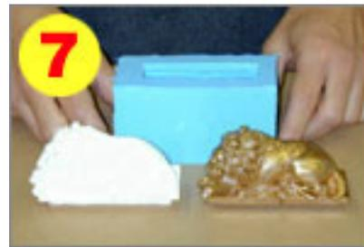
Depending on working temperature, humidity, and catalyst type, your mold will be ready in between 6 and 24 hours. Higher temperature and humidity accelerate the cure. Even though the mold may be usable right away, it continues to cure for a full week. The best castings will be produced after this full cure time, especially if casting in polyester. Quick-Cast is shown in this picture.
