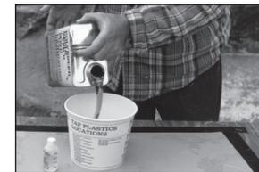
Mix resin and catalyst on a clean flat working surface near the area to be glassed. Stir vigorously, scraping sides of container and lifting resin from the bottom (use a motion like
