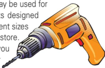
When drilling a hole three times deeper than the diameter of the drill, a lubricant, or coolant should be used, such as water. This will help remove chips, dissipate heat, and improve the finish of the hole. Rough, irregular, or fuzzy holes can lead to cracking and breaking months after the piece has been completed.
