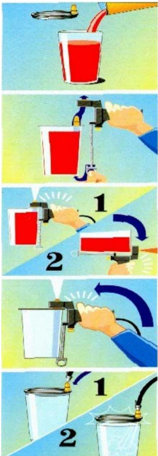
1. Fill the cup with gelcoat and catalyze according to the material supplier's specifications. Do not overfill beyond the 1000cc level, as this will cause leakage from the vent hole. Be sure the vent hole is not clogged. This will greatly effect the spraying action of the gun.
