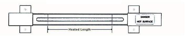
All Free-Standing Heating Trays run on standard 120 volts and have a maximum operating temperature of 800°f. Units can be used with the below-listed Power Controls where temperature control is desired.
