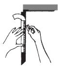
Spray Film and firmly squeegee surface to remove excess water between film and glass. Using paper towels blot edges of film completely dry.
