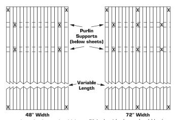
48 inch wide sheets should be fastened to supports at all four corners, and at points 6" in from the edges of each purlin support.
