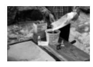
Thicken final color coat of resin with TAP Visco-Fill or Cab-O-Sil. The consistency of this mixture should be creamy enough to hang on a vertical surface and to fill
