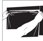
Use the Squeegee to apply film to the window, working from the center of the film to the outer edges with short gentle strokes. Carefully work out wrinkles and bubbles with the squeegee. Do not squeegee all the way to the edge yet. Leave about 1" all the way around.
