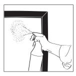
**Clean Finished Window** with a non-ammoniated window cleaner *(your soap-solution is ideal).* When you clean the window, be careful not to disturb the film's adhesion to the glass—it will not bond completely until it is dry, which can take up to 30 days depending on sun exposure.
