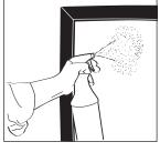
Apply Film In Place with the adhesive side on the window. The soap solution acts as a lubricant to allow positioning of film. GENEROUSLY spray "room-side" surface of film to lubricate before squeegeeing.
