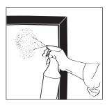
**Clean Finished Window** with a non-ammoniated window cleaner *(your soap-solution is ideal).* When you clean the window, be careful not to disturb the film's adhesion to the glass—it will not bond completely until it is dry (it will take several days).
