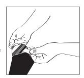
Spray Soap Solution generously over entire window surface. Avoid spraying the edge of the glass as this can wash trapped dirt onto the glass. Next spray adhesive side of film with the soap solution (the side exposed by removal of liner).
