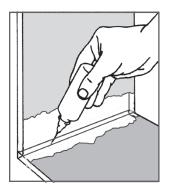
should be applied with a **TAP Hypo-Applicator**. The cement will flow into the joint through capillary action. The union will 'set' quickly, firm enough to proceed with your work, and will reach high strength in 24-48 hours. Edges should not be flamed or polished prior to gluing, this could result in the edges crazing.
