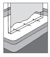
provides an air-free cushion when the two pieces are joined together. (Do not allow Acrylic Cement to contact the face of the sheet.) The result is an ideal bond that becomes as strong as the sheet itself. It takes up to twenty-four hours to cure the joint.
