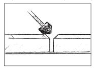
**6.** Let the filler (compound or mixture) begin to cure. Before complete cure, remove the tape and use the surform file to remove high spots and create a slightly concave
