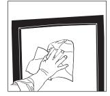
foreign matter. Spray the window with a liquid soap solution (soap solution: 1 tsp of clear liquid shampoo, i.e. Johnson's Baby Shampoo, per qt of water). Scrape entire wet window surface with the Window Scraper to remove foreign debris. Use the soap solution again, scrub the window with a sponge, and squeegee window clean. MEASURE your window and cut film approximately 1" to 2" wider and 1" to 2" longer than window.
