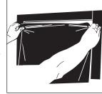
Use the Squeegee to apply film to the window, working from the center of the film to the outer edges with short gentle strokes. Carefully work out wrinkles and bubbles with the squeegee. Do not squeegee all the way to the edge yet. Leave about 1" all the way around.
